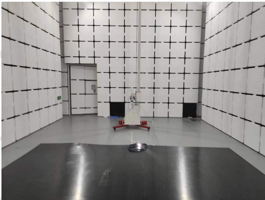
Photo 6 Radiated Emission Test
