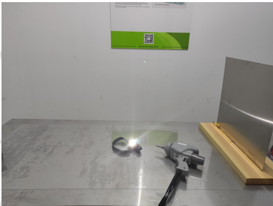
Photo 8 Electrostatic Discharge Test
